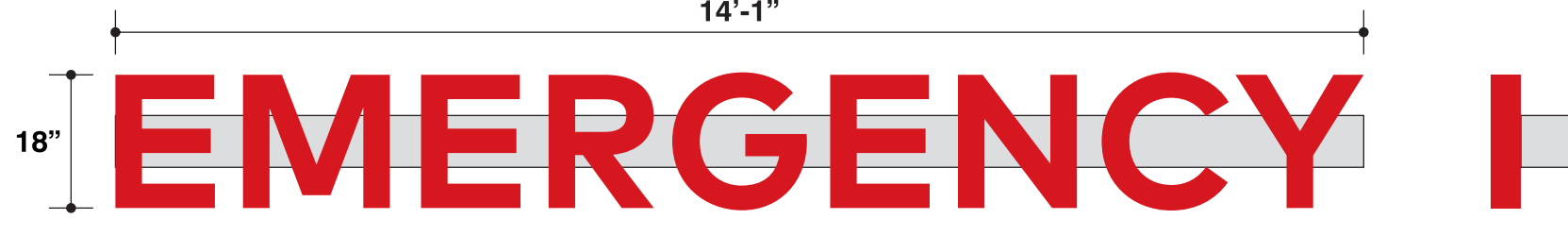
C ELEVATION DETAIL - EMERGENCY DEPARTMENT CANOPY @ ENTRANCE - SIGN LOCATION - EXT-01 SCALE: 1/4" - 1'-0"
