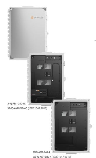
The IQ Combiner 4/4C with IQ Gateway and integrated LTE-M1 cell modem (included only with IQ Combiner 4C) consolidates interconnection equipment into a single enclosure. It streamlines IQ Microinverters and storage installations by providing a consistent, pre-wired solution for residential applications. It offers up to four 2-pole input circuits and Eaton BR series busbar assembly.
