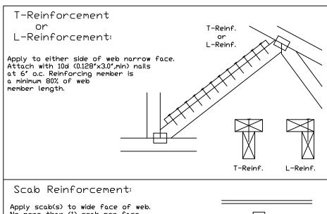
Apply scab(s) to wide face of web. No more than (1) scab per face. Attach with 10d (0.128"x3.0",min) nails at 6" o.c. Reinforcing member is a minimum 80% of web member length.
