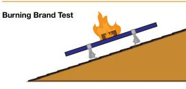
A burning wooden block is placed on module as a fan blows at 12 mph. Flame cannot be seen on underside of roof within 90 minutes.
