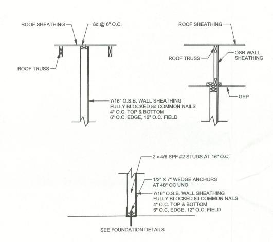
INTERIOR SHEAR WALL DETAIL
