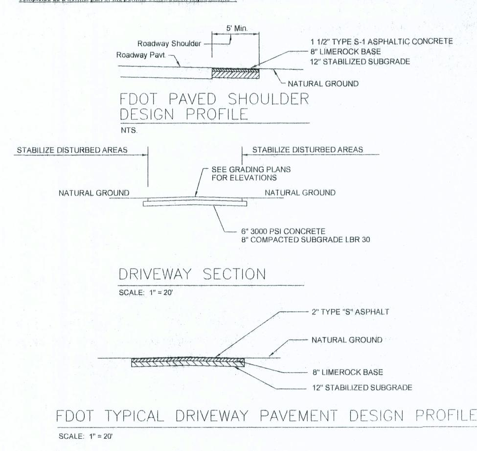
IF CONCRETE IS USED, A MINIMUM POURED THICKNESS DEPTH OF 8 INCHES THE FIRST 5 FEET FROM EXISTING ROADWAY PAVEMENT EDGE WITH A MINIMUM 6 INCHES DEPTH THEREAFTER TO THE R/W LINE IS REQUIRED. CONCRETE SHALL HAVE A MINIMUM 28 DAY COMPRESSIVE STRENGTH OF 3000 PSI.
